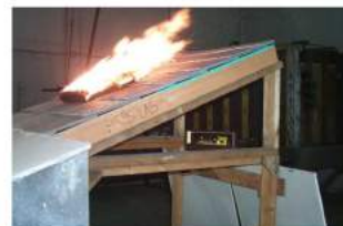
Test to determine the fire rating for a roof covering. A Class A burning brand is on this roof covering. Photo taken during experiments conducted at the University of California Fire Research Laboratory. Source: Stephen L. Quarles
